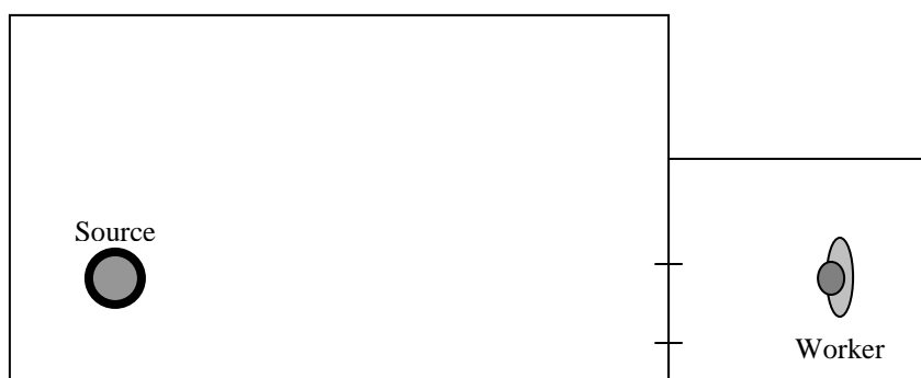
Figure 3.6.2 Complete personal enclosure (doors and windows closed)
