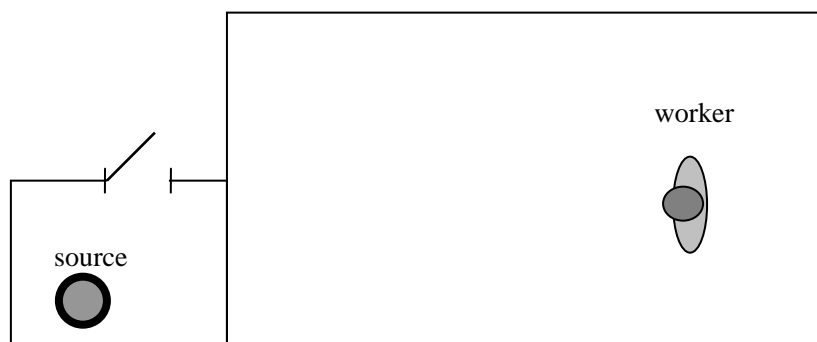
Figure 3.5.4 No segregation (source is in another department)
