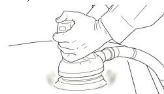
On-tool extraction (HSE, 2008)
