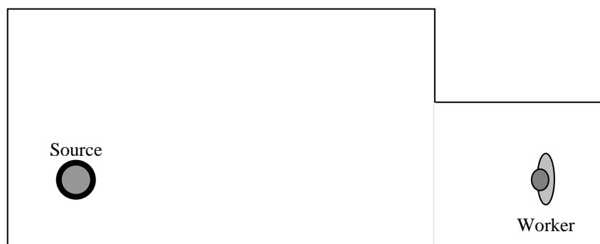
Figure 3.6.5 No personal enclosure (opening between worker and source is larger than a door or window)
