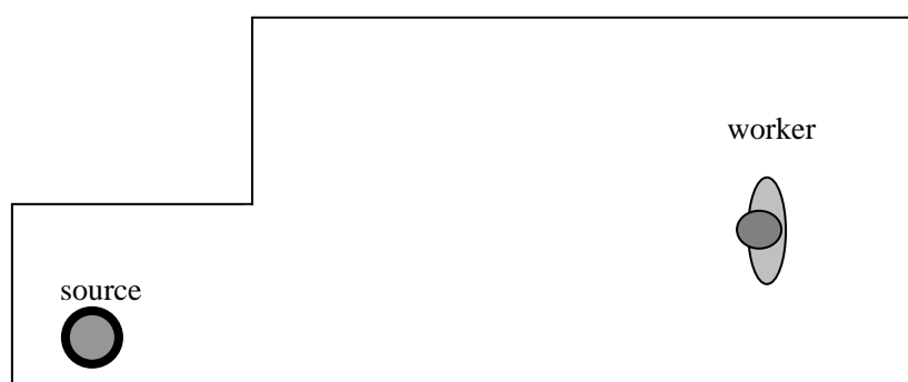
Figure 3.5.5 No segregation (opening between source and worker is larger than a door or window)
